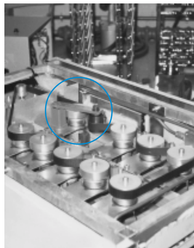
Flat belt drive with tensioning element type SE and tensioning roller type R
